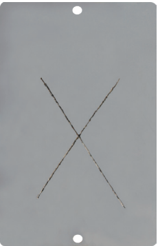
单边腐蚀 Single side corrosion 1.6mm
