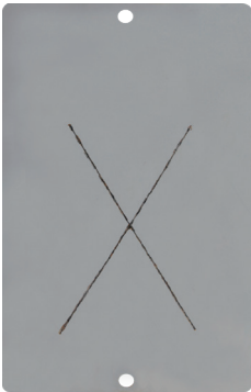
单边腐蚀 Single side corrosion 1.3mm
