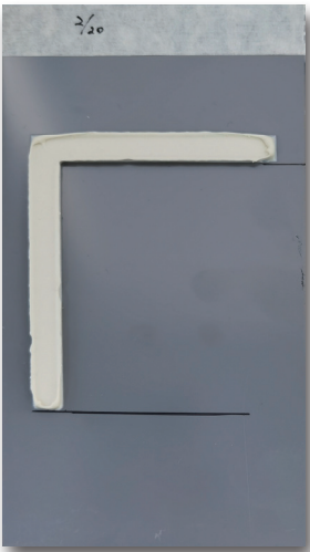
密封胶抗流挂和附着力测试优良 Sealant anti-flow hanging and adhesion testing is excellent
