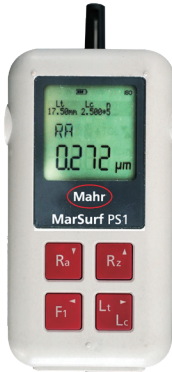
粗糙度测试仪测量 0.272μm The roughness tester measures 0.272μm
