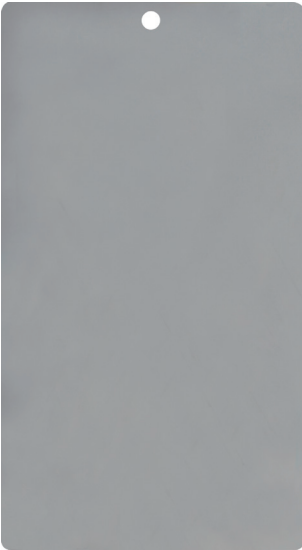
粗糙度测试仪测量 0.272μm The roughness tester measures 0.272μm
